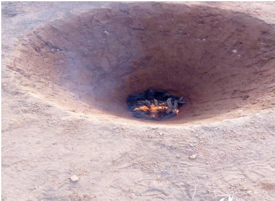
Figure 5 Beginning of pyrolysis process
